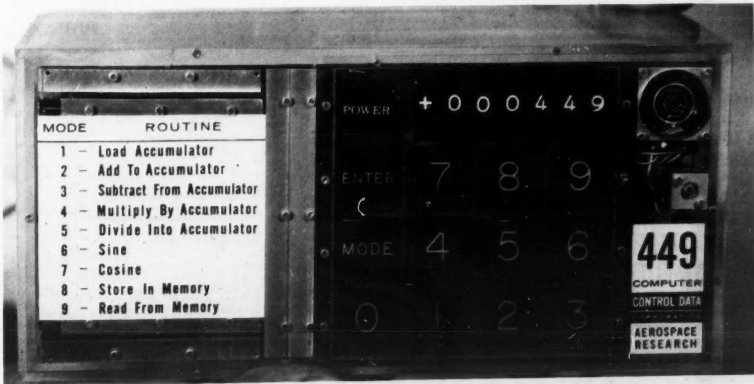
The Control Data 449 computer system claims to be the world's smallest electronic computer. Measuring 4" x 4" x 9", the outer
